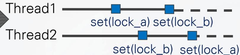
**// Thread1 waits for lock\_b owned by Thread2, whereas Thread2 waits for lock\_a owned by Thread1. Thus, neither thread can free a lock and both threads wait indefinitely.**
